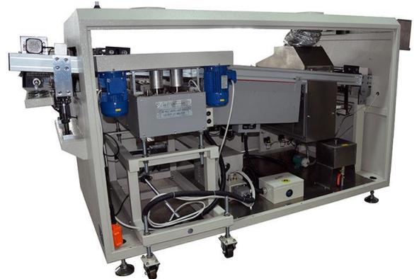
The specially designed, heavy duty guiding rails reduce the deformation caused by heat; After two years working you only need to change the cooper bars instead of change the whole conveyor rails.
