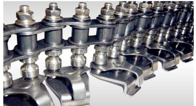
Optional with heavy load Titanium fingers (5mm) to transport PCBs/Pallets of up to 20 kgs per unit
