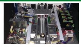
H351: 5 axis combined controller for X,Y,Z, R,and solering wire feeding motion system.
