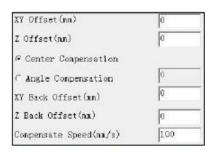
The machine will calculate compensation spots automatically if the compensation data have been setup, and there is no need for manual spot selection.
