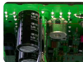
Mixed PCB, tall components beside soldering pad
