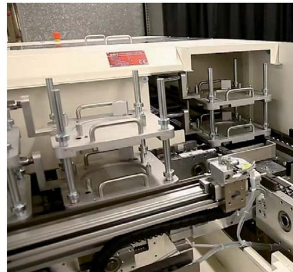
These heavy load systems are designed for transporting and handling assemblies and components with a total weight of up to **9 kg per meter**. Higher weight available on request.
