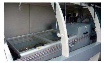
The heaters can be drawn out of the rear of the machine and the blowers can be taken out at the top of the zones making maintenance easy and fast
