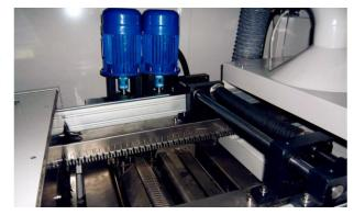
Optional In-loading system: which can connect with the insertion conveyor directly, the sensor at bottom for counting and spray fluxer on/off; with ruler and needle for instruction of width.
