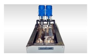
Dual wave solder. Both wave heights are controlled by transducer. Changing the wave height is controlled by adjusting the frequency of power. High quality wave motors made in Italy.
