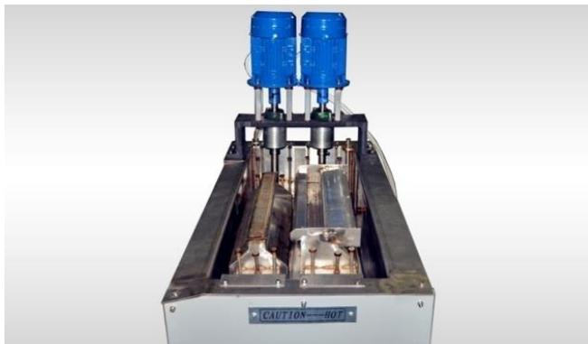
Dual wave solder. Both wave heights are controlled by transducer. Changing the wave height is controlled by adjusting the frequency of power. High quality wave motors made in Italy.
