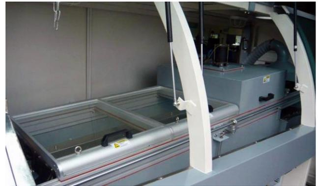
Optional to add 3rd upper preheating zone, minimize the PCB up/bottom side temperature difference and reduce the board deformation.
