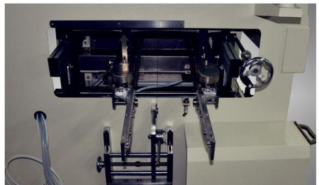
Standard equipped with 3 hot air convection preheating zone at bottom, provide enough heat to active the flux performance.
