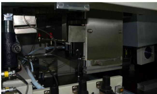
Japanese made sprayer for perfect atomization performance of the flux unit. Fully programmable and driven by stepper motor for precise spraying applications.
