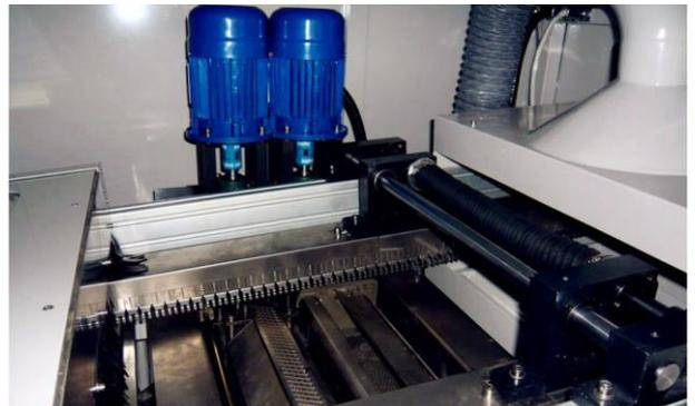
Optional In-loading system: which can connect with the insertion conveyor directly, the sensor at bottom for counting and spray fluxer on/off; with ruler and needle for instruction of width.
