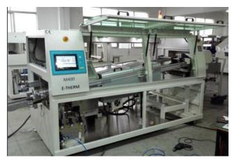
The specially designed heavy duty guiding rails reduce the deformation caused by heat; After two years working you only need to change the cooper bars instead of change the whole conveyor rails.
