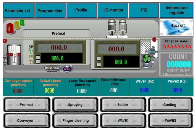
The software include all functions like PCB counting, temperature setting and editing, PCB parameter menu, and profile testing, alarms, control of motor temperatures as well as Multilanguage support.
