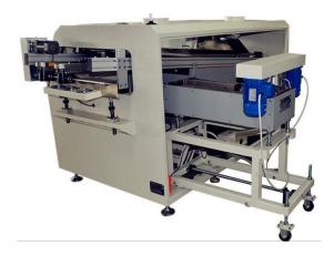
Solder pot can lift up and down, move in and out automatically. Ideal changing the solder pot for different applications and the conversion between leaded and lead-free.
