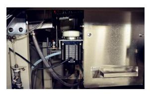
Japanese made sprayer for perfect atomization performance of the flux unit. Fully programmable and driven by stepper motor for precise spraying applications.
