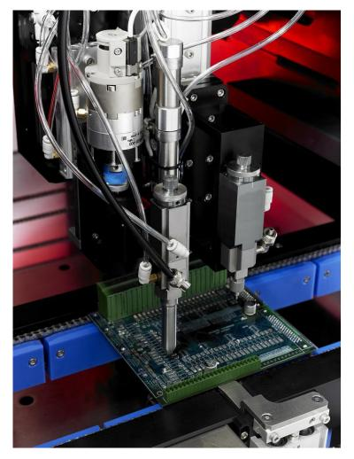
Stand equipped with stainless steel chain conveyor and automatic width adjustment mechanism.
