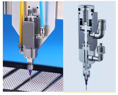
Microdot needle valve SY-420 is designed for precise dispensing of mid and low viscosity fluid, such as silicone oils and UV-cure adhesives. It is a kind of pneumatic and flow adjustable needle valve, which used in precise microdot dispensing. It's septum made from High molecular weight polyethylene (UHMW PE), departs fluid slot and operation components. So it is elaborate and durable. Shut off the tip inside the stainless steel needle, which guarantees no remains.
