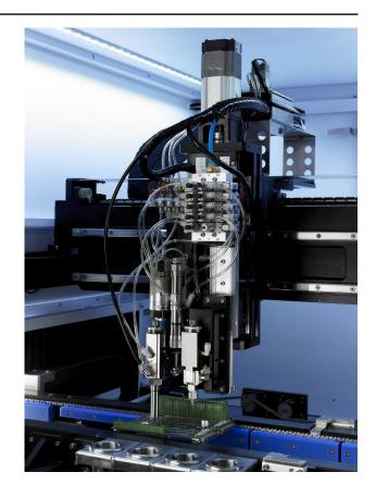
Panasonic servo motor and driving system make the position repeatibility can reach 0.05mm, high speed response and movement.
