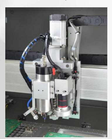
Quality, air cooling routing spindle for a long life time
