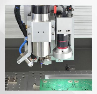
Equipped with anti static ionizing air gun which keep cutter clean when operating
